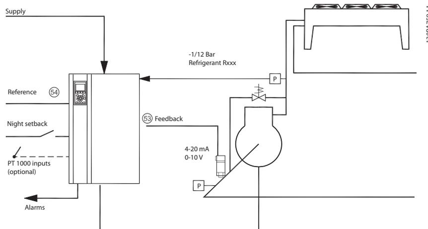
Illustration 6.1 Standard Drawing of "Compressor with Internal Control"
