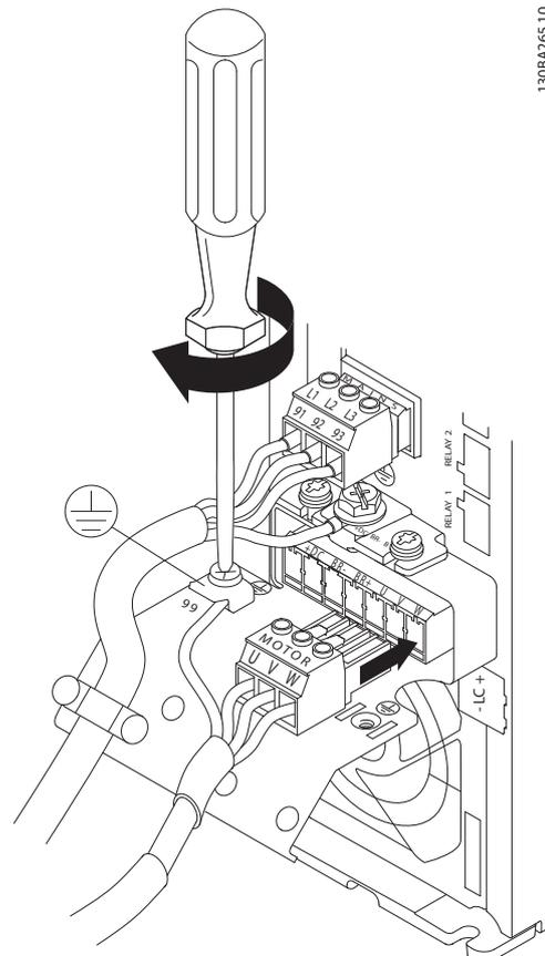
Illustration 2.13 Motor Connection for A2 and A3
