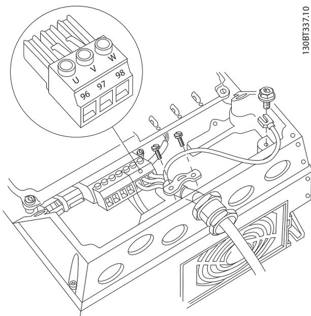
Illustration 2.15 Motor Connection for A4 and A5
