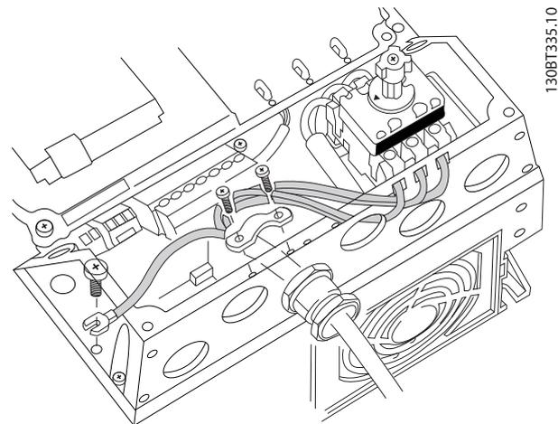
Illustration 2.24 Connection to Mains and Earthing with Mains Disconnect Switch
