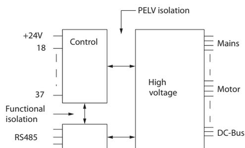
**Illustration 10.1 PELV Isolation of Analog Inputs**
