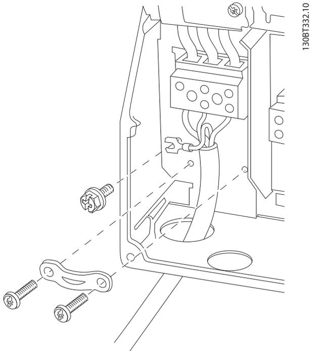
Illustration 2.25 Connection to Mains and Earthing for B1 and B2
