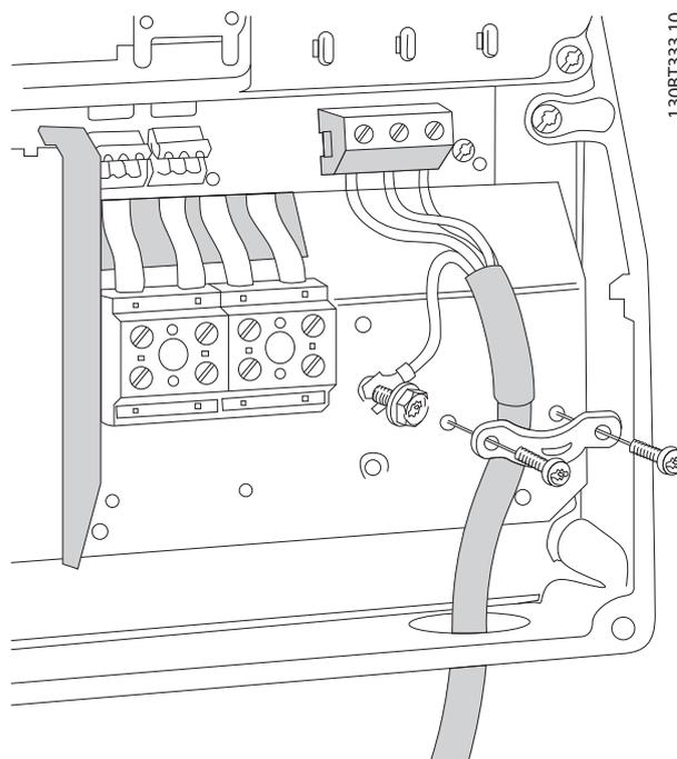
Illustration 2.16 Motor Connection for B1 and B2
