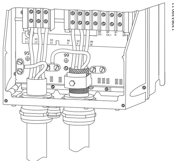
Illustration 2.17 Motor Connection for C1 and C2
